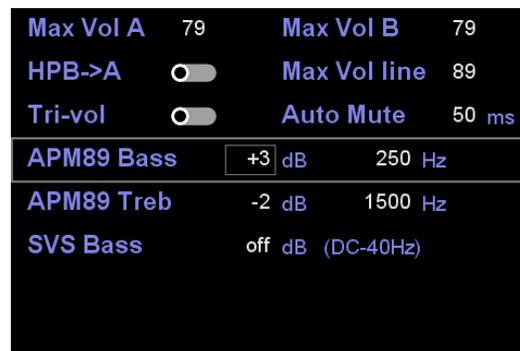
For consistency, the SVS bass shelving filter control has been moved to MISC SETTINGS. Note that SVS Bass operates on the headphone signal (output from the SVS processors) whereas the APM89 Bass/Treb operates on the audio input to the SVS processors and the audio output to the line outputs in AV mode.
